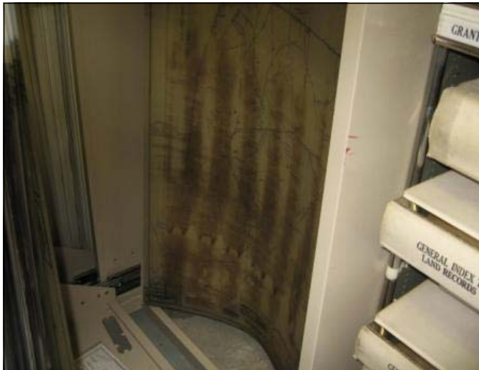
Image 2: Brown or tan streaks are one typical sign of deterioration in fixed line maps.
